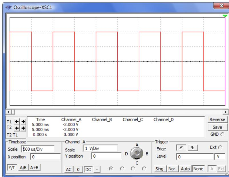
13. For each of the two digital signals shown below, determine the amplitude, period (T), frequency (F), time high ( $t_H$ ), time low ( $t_L$ ), and duty cycle (DC). Be sure to put your answer in proper engineering notation and use the correct units.
