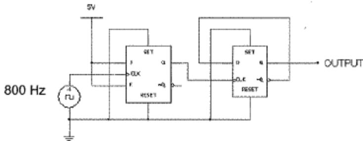
For the 74LS76 J/K flip-flop shown below, complete the timing diagram for the output signal Que. Note that the CLK input for this flip-flop is a negative edge trigger and both the PR and CLR asynchronous inputs are active low.
