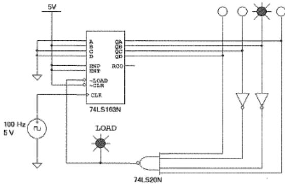
37. Determine the output frequency for the circuit shown below.
